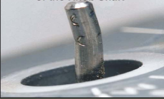
FIGURE F2 Shows double bending of the Knob Shaft
